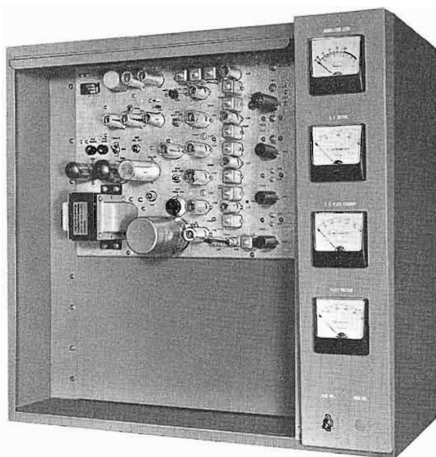
Front view (cover removed) of Model BFE-10C, ten watt FM transmitter. Models BFE-50C and BFR-50C are essentially the same in appearance.
